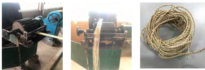
Fig 2. (a) Inserting banana pseudo stem to the decorticator, (b) extracted banana fibers and (c) hand-spun banana yarns
