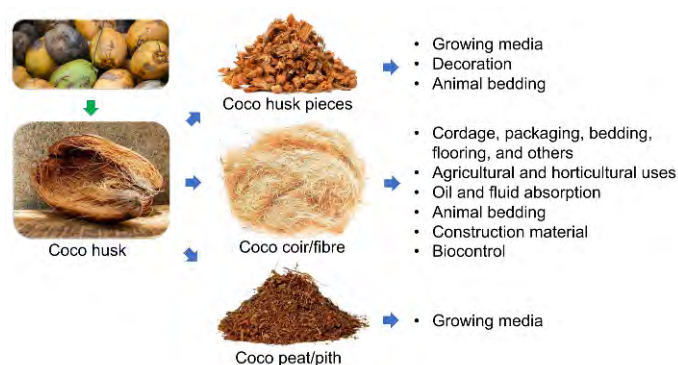
Fig 1. Derivation of by-products of the Coconut extraction process and its commercial use
