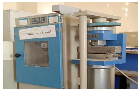
Fig.7 Flexural strength test machine.
