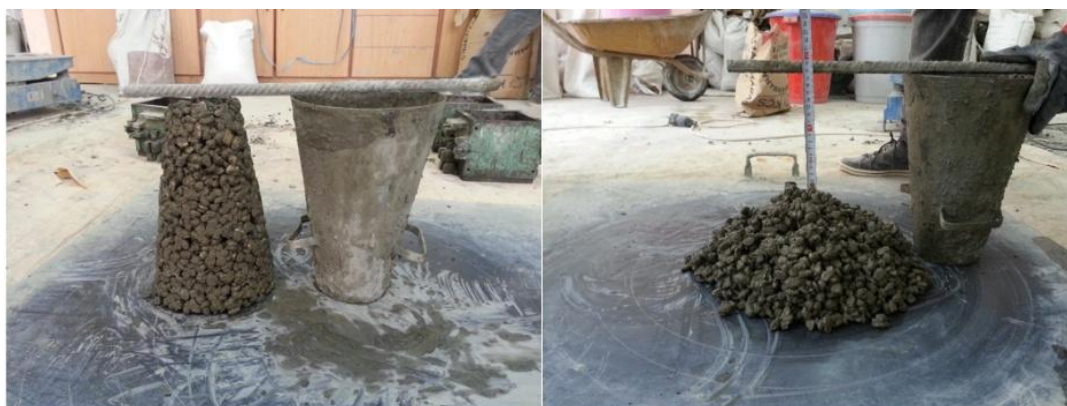
Fig. 1 Samples of pervious concrete with dissimilar W/C relations, slump test
