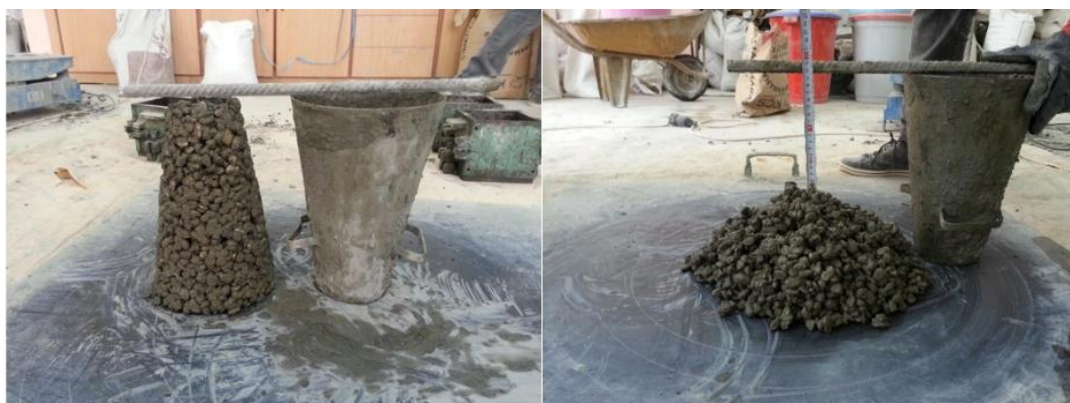
Fig. 1 Samples of pervious concrete with dissimilar W/C relations, slump test
