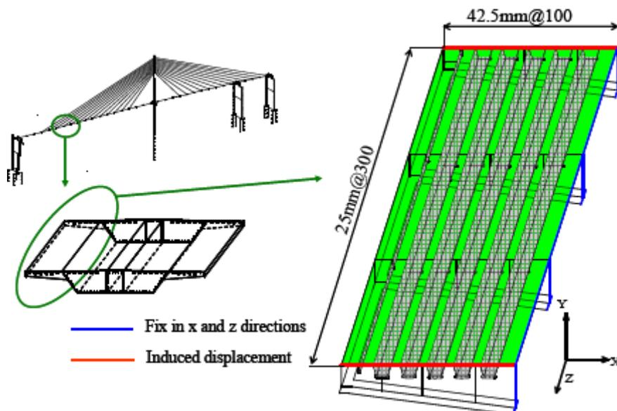
Fig. 10 Analytical model of steel deck system for Finite Element Analysis.
