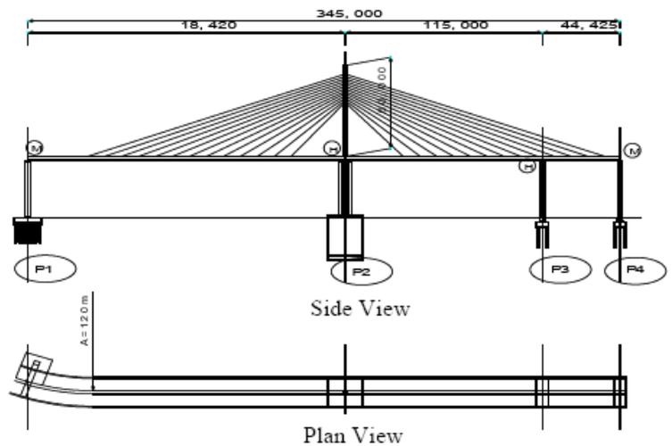
Fig. 5 Target cable-stayed bridge (named Aratsu bridge) (unit:mm).
