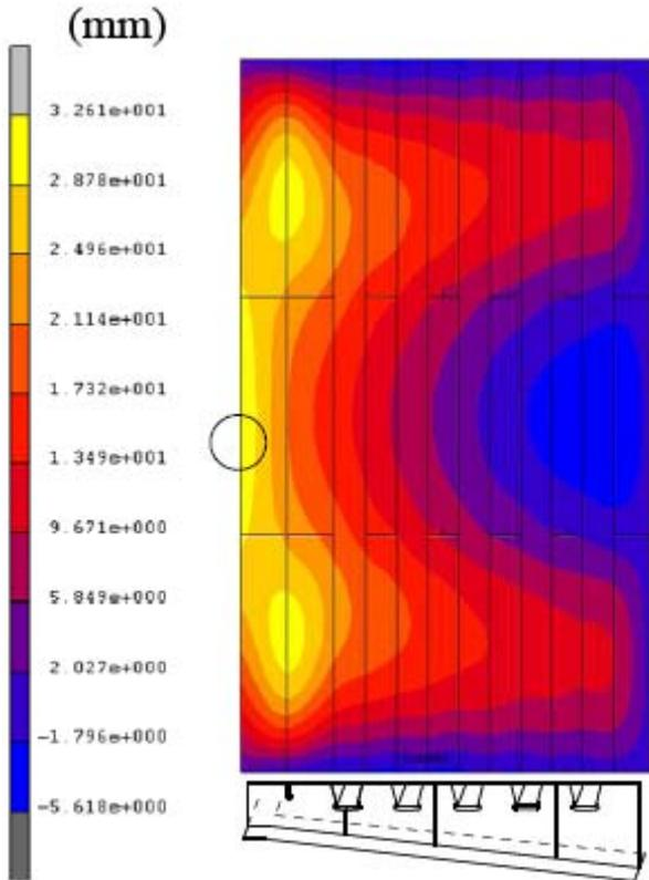
Fig. 10 Distribution of maximum vertical displacement of deck plate when 2 yield-strain is induced at edge of mid span plate (circle point).
