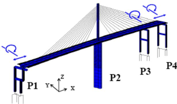
Fig. 6 Image of analytical model (Frame Structure).
