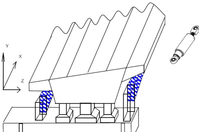
Fig. 7 Image of damper installed at girder end and sketch of velocity proportion damper.
