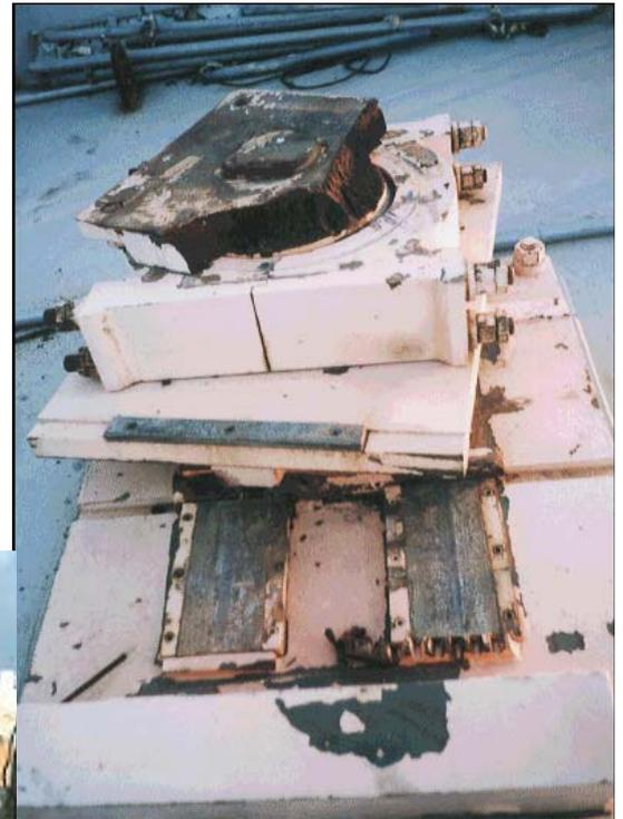
Fig. 3 Failure example of pivot roller support.
