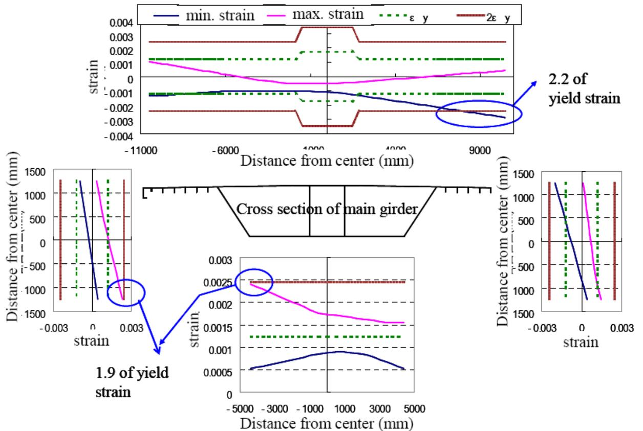
Fig. 9 Strain distribution on main girder.
