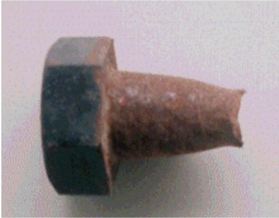
Fig. 2 Failure configuration of a set bolt.
