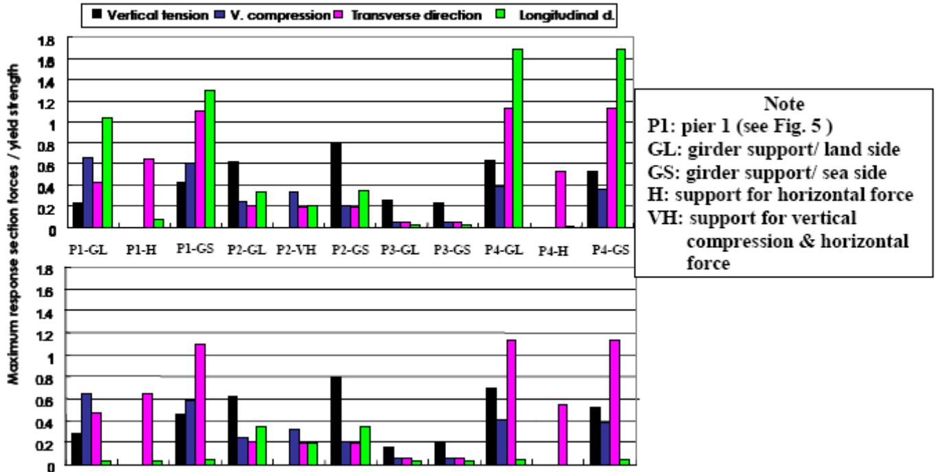
Fig. 8 Comparison of response section forces before (upper) and after (below) retrofit.
