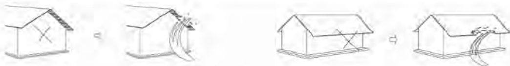
try to avoid this roof cantilever/canopy
