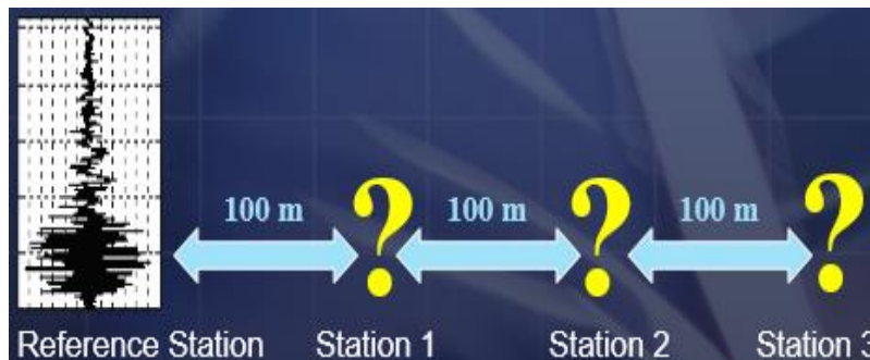
Fig. 2 A Schematic of Conditional Simulation with Four Points Aligned at 100 m Intervals, Starting from reference station
