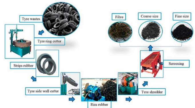
Fig. 5 Methods of preparing tire rubber fibers (M. Mhaya et al., 2021)
