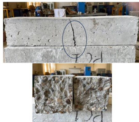
Fig. 15 Failure of a prism sample containing walnut shells after the flexural strength test
