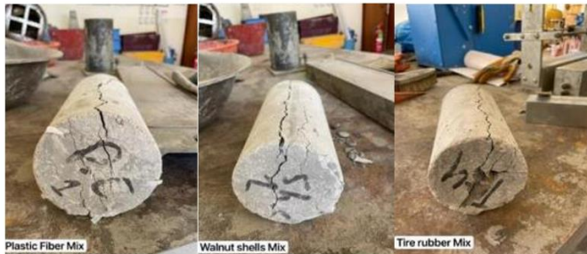
Fig. 12 Failure of cylindrical samples containing different waste materials after the splitting tensile strength test
