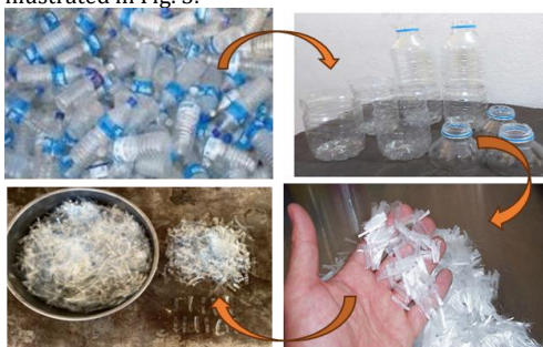
Fig. 3 Process of making plastic PET fibers
