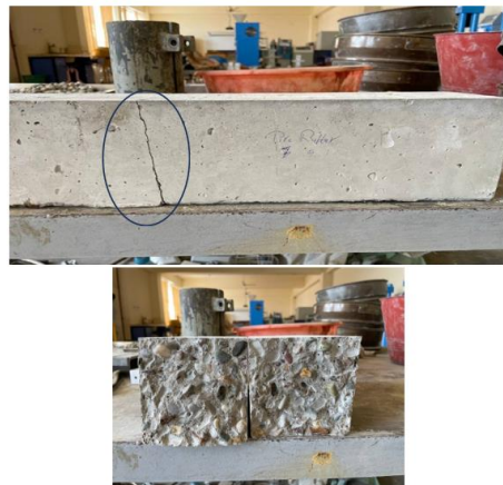
Fig. 16 Failure of a prism sample containing tire rubber after the flexural strength test
