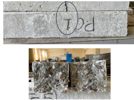
Fig. 14 Failure of a prism sample containing PET plastic fibers after the flexural strength test
