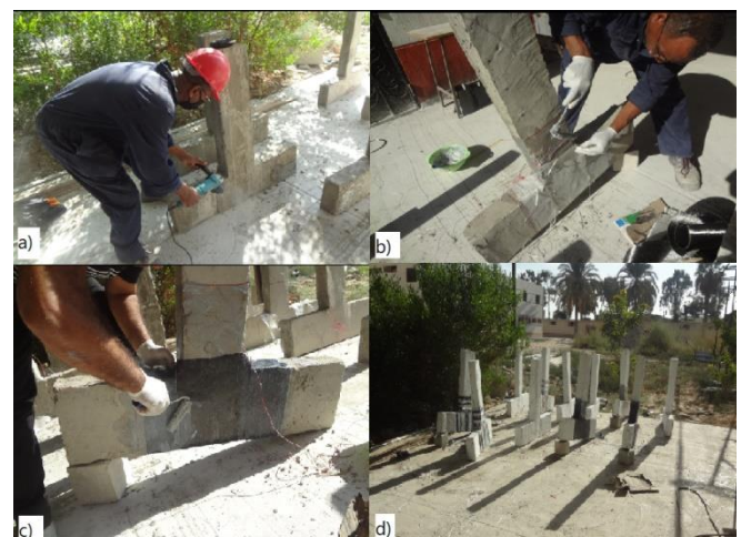
Fig. 7 Preparation and processing strengthening specimens: a) Surface leveling, b) applying primer epoxy layer on surface and installing the FRP sheets, c) Resin putting on FRP sheet, d) placing the strengthened beam column joints for curing
