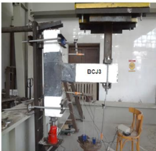
Fig. 9 Photo of the loading arrangements and instrumentation
