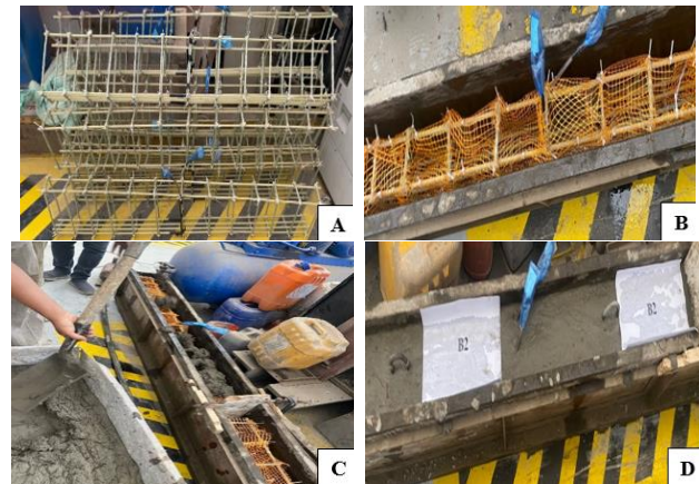
Fig. 2 Preparation and casting processes.
