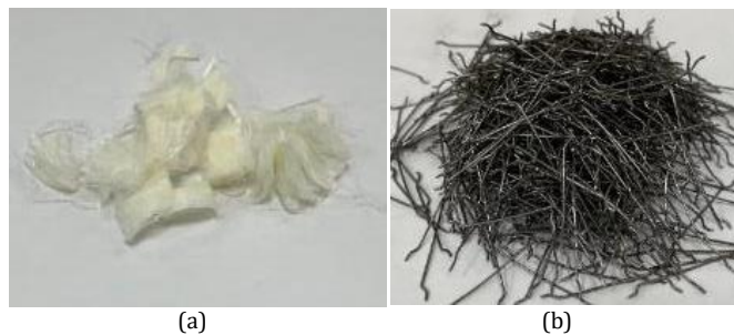
Fig. 2 Hybrid Fibers (a) Polyacrylonitrile fiber; (b) Steel fiber
