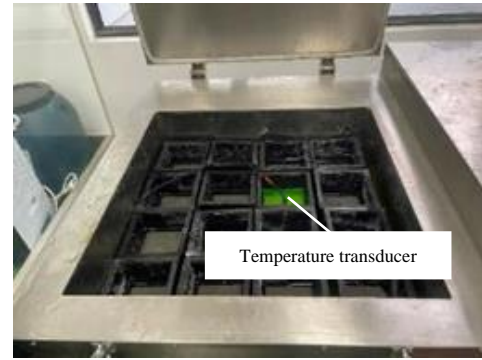
Fig. 4 Rapid Freeze-Thaw Test
