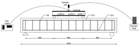
Fig. 8 The illustration of experiment setup
