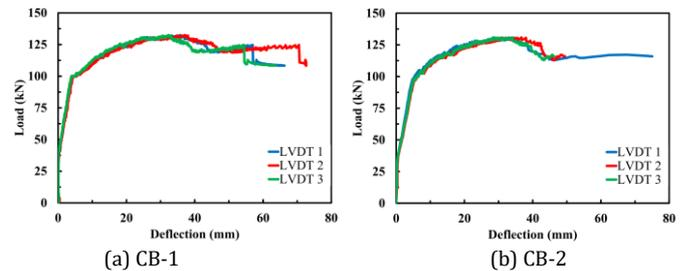
Fig. 10 Load VS Deflection Graphs for CB
