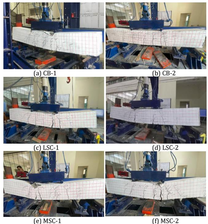
**Fig. 13 Flexural crack pattern on beam specimens**
