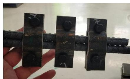
Fig. 4 Clamp connector used in this research
