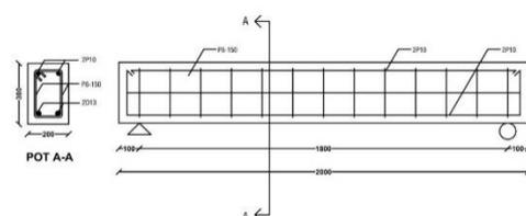
Fig. 5 Detail reinforcement of RC beam without rebar splicing (CB)
