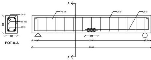
Fig. 7 Detail reinforcement of RC beam with mechanical splice (MSC)
