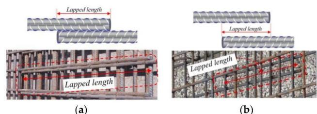
Fig. 1 Lap splice (a) contact (b) non-contact (Fayed et al., 2023)
