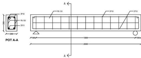
Fig. 6 Detail reinforcement of RC beam with lap splice (LS)
