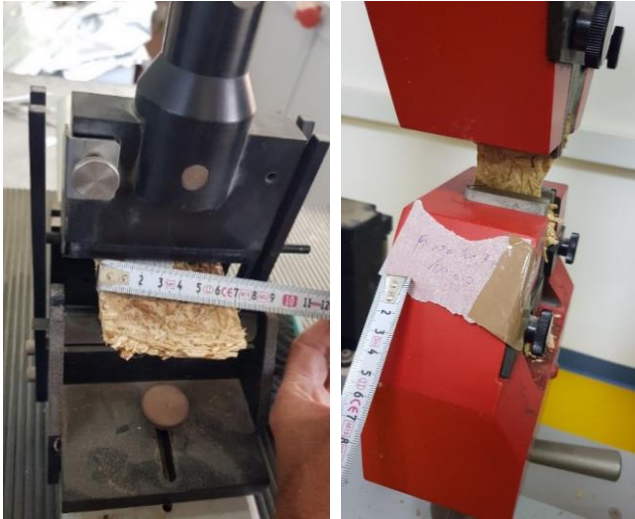
Fig. 3 photos of the spruce chipboard sample tensile (Right) and bend testing (left).
