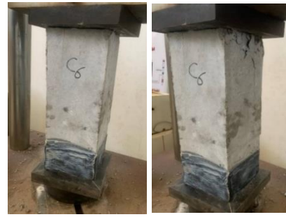
Figure 11. Cracks Pattern for Column with CFRP at the bottom base.
