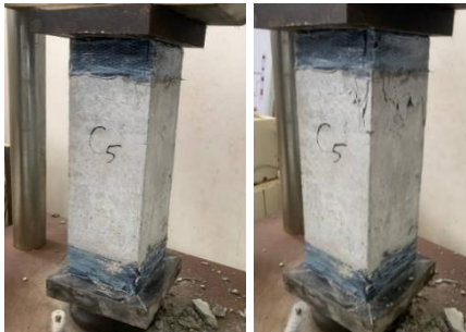
Figure 10. Cracks Pattern for Column with CFRP at the top and bottom base.
