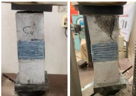
Figure 9. Cracks Pattern for Column with CFRP at the mid span
