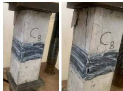
Figure 13. Cracks Pattern for Column with CFRP at the mid span (100 mm width) under repeated 30% ultimate load)
