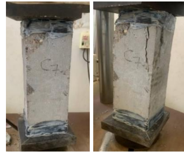
Figure 12. Cracks Pattern for Column with CFRP at the upper and lower base (50 mm width) under repeated 30% ultimate load
