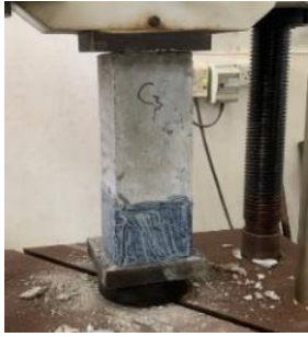
Figure 8. Cracks Pattern for Column with CFRP at the lower base
