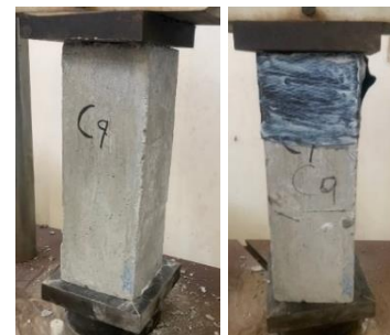
Figure 14. Cracks Pattern for Column with CFRP at the upper base (100 mm width) under repeated 30% ultimate load
