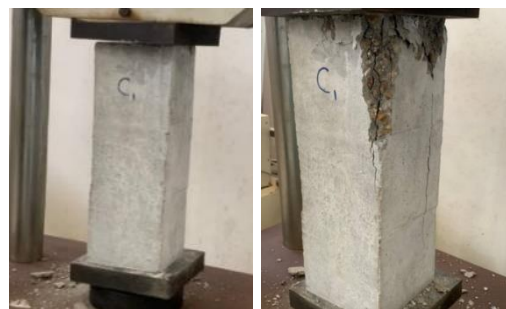
Figure 6. Cracks Pattern for Column Without CFRP (Control)
