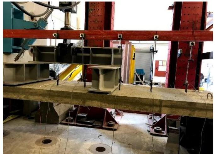
**Fig. 7 UBSR1 specimen with the LVDTs fixed in their positions**
