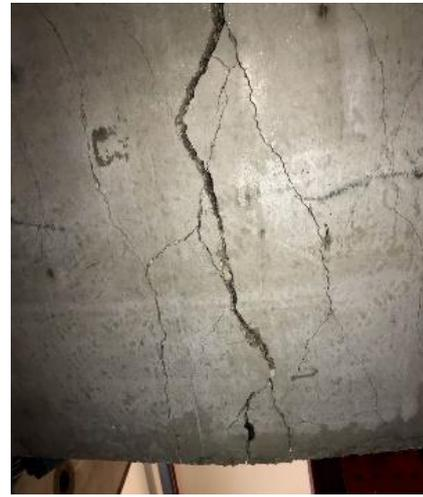
**Fig. 10 Cracks formed at UBSR2's bottom surface**
