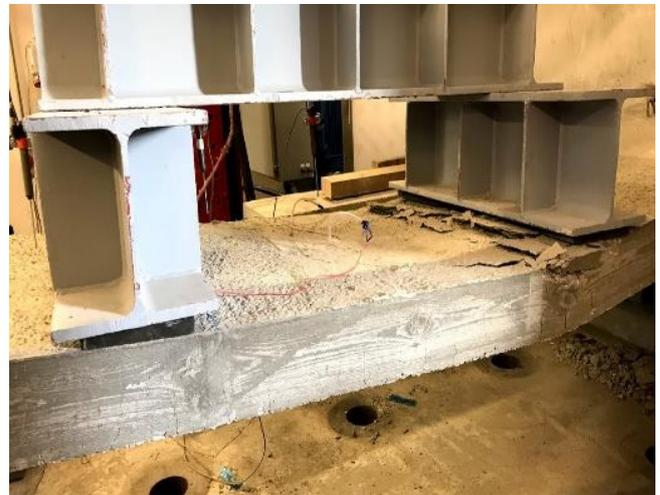
**Fig. 12 UBSR2 after failure at the location of the loading beam**
