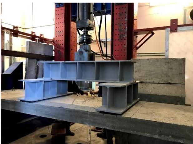
**Fig. 6 The full setup of one of the specimens showing the rubber pads located between the loading beams and the specimen**
