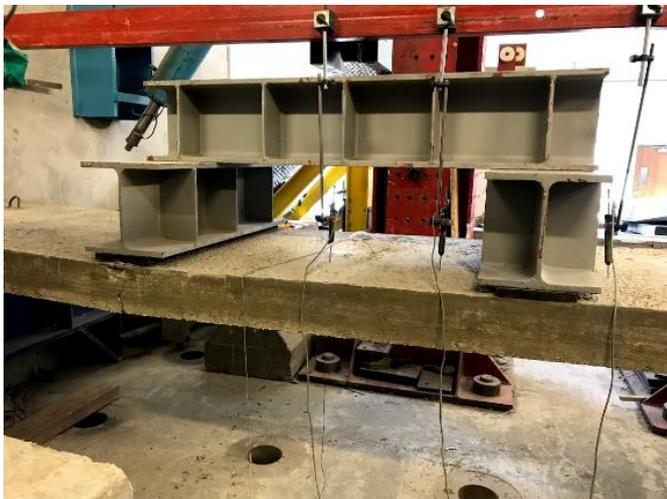
**Fig. 9 UBS2 after failure and unloading**
