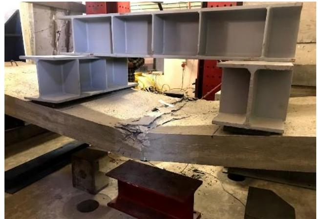
**Fig. 11 UBSR1 after failure at mid-span**
