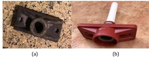
Fig. 2 (a) Anchor for the bonded system, provided by Strands Company, Egypt. (b) Encapsulated Anchor for the Unbonded System, provided by GTI, USA.
