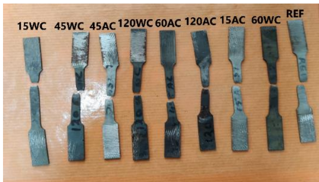
Fig. 11 Failure pattern of the coupon specimens tested.
