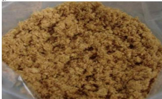
Fig. 1 Bamboo pulp fiber
