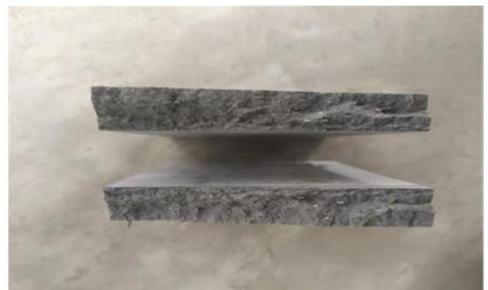
**Fig. 10 Bending failure form of PFRCC pane**
