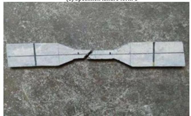
(b) Specimen failure form 2
