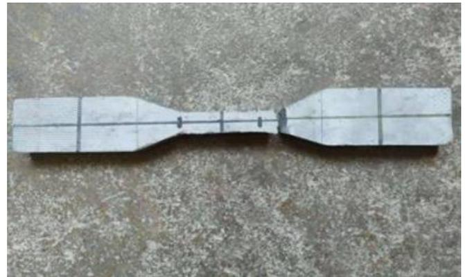
(a) Specimen failure form 1
