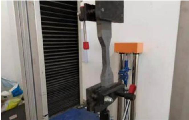
Fig. 4 Axial tensile test of PFRCC panel
