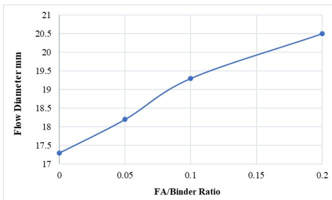
**Figure 2. The influence of FA/Binder on the geopolymer concrete Flow Diameter (mm).**
