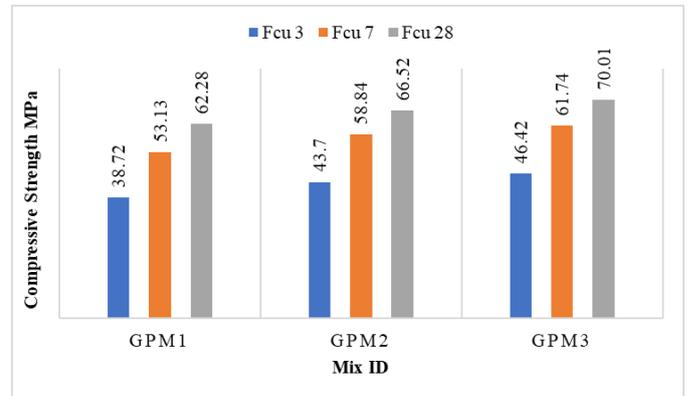
Figure 5. The influence of alkaline\binder on the geopolymer concrete compressive strength (MPa).
