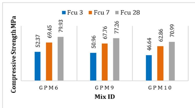
**Figure 8. The influence of sand B/sand A on the geopolymer concrete compressive strength (MPa).**
