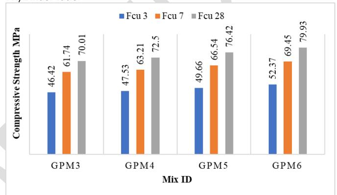
Figure 6. The influence of FA/Binder on the geopolymer concrete compressive strength (MPa).
