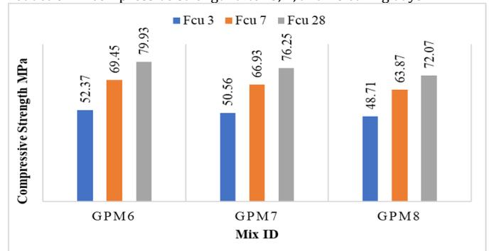
Figure 7. The influence of sand/binder on the geopolymer concrete compressive strength. (MPa).
