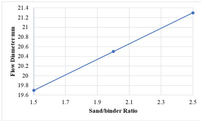
Figure 3. The influence of sand/binder on the geopolymer concrete Flow Diameter (mm).
