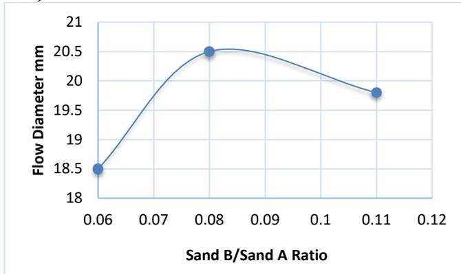
Figure 4. the influence of sand B/sand A on the geopolymer concrete Flow Diameter (mm).
