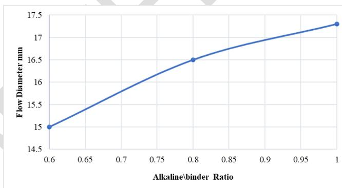
**Figure 1. the influence of alkaline\binder on the geopolymer concrete Flow Diameter (mm).**
