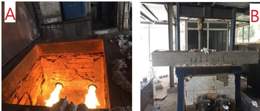
Figure 5 - a. The Fire Furnace, b. fire setup for beam.
