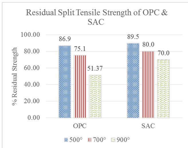
Figure 10. Percentage Residual Split Tensile Strength
