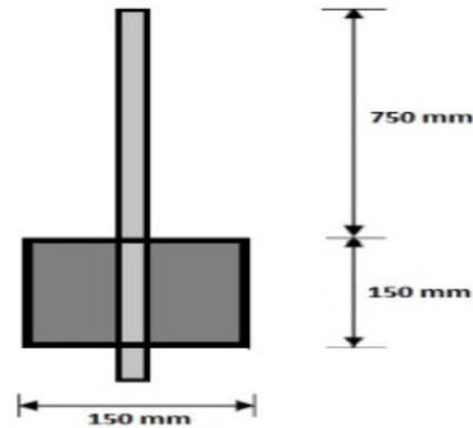
Figure 1. Bond test specimen
