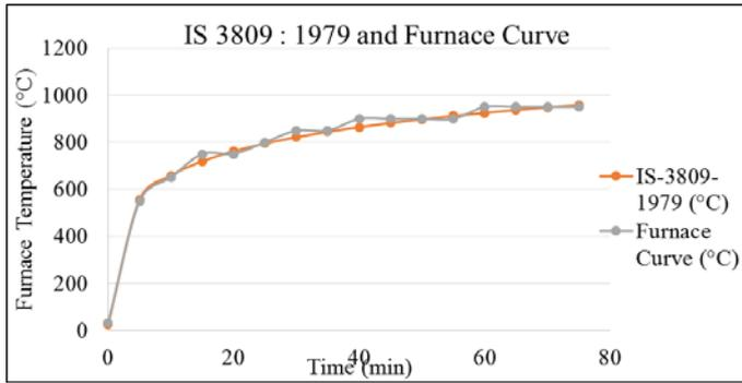
Figure 3. Comparison of IS: 3809:1979 recommended curve & Experimental curve
