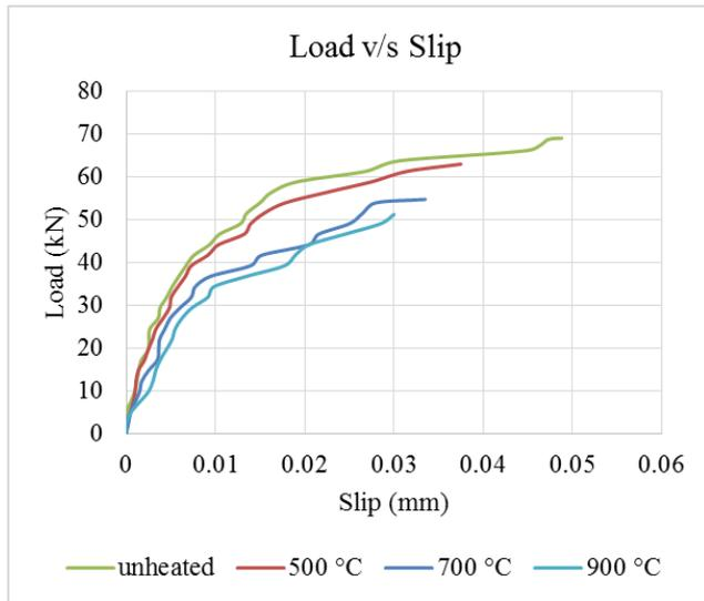
Figure 12: Load v/s Slip graph for SAC
