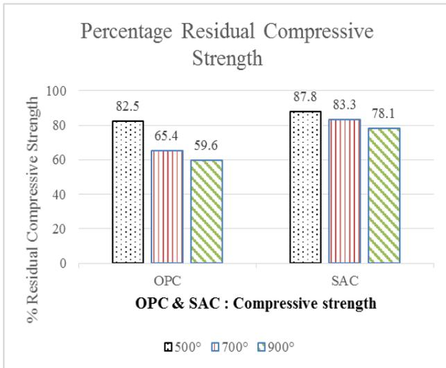
Figure 6. Percentage residual Compressive strength
