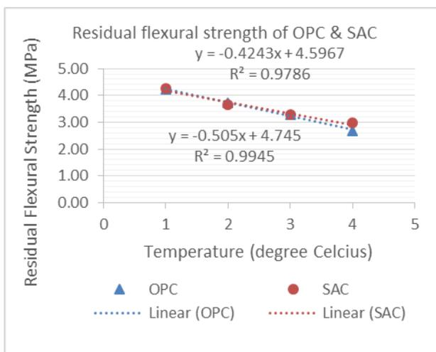
Figure 7. Reduction in Flexural Strength for OPC and SAC
