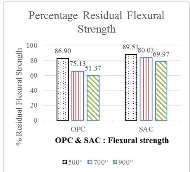
Figure 8. Percentage Residual Flexural Strength of OPC and SAC.
