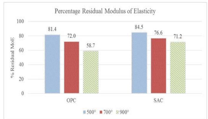
Figure 11: Residual Modulus of Elasticity for OPC and SAC
