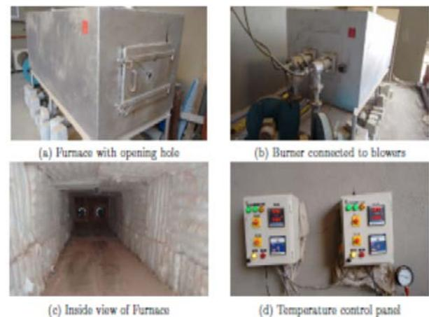
Figure 2. Furnace used for application of high temperature
