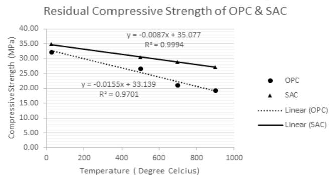
Figure 5. Change in compressive strength at different temp ranges.
