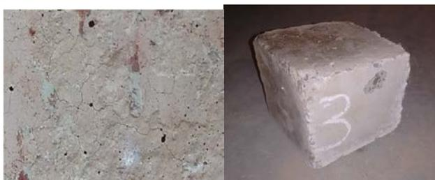
Figure 4. a) Cracks in SAC 4 b) Spalling in OPC
