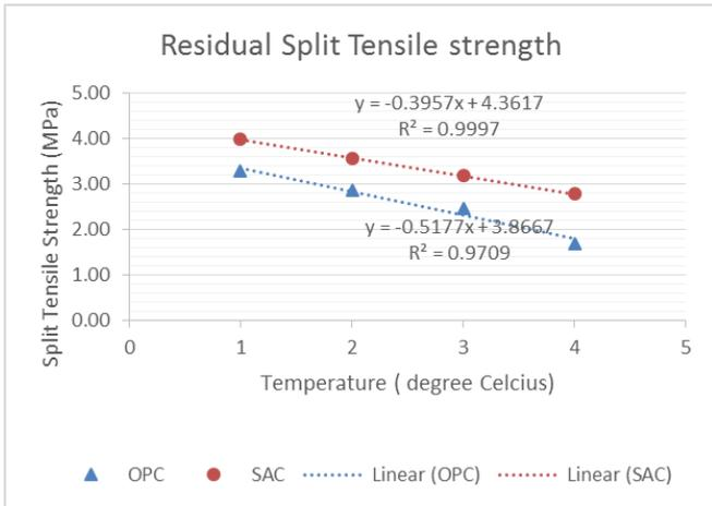
Figure 9: Reduction in split tensile strength.
