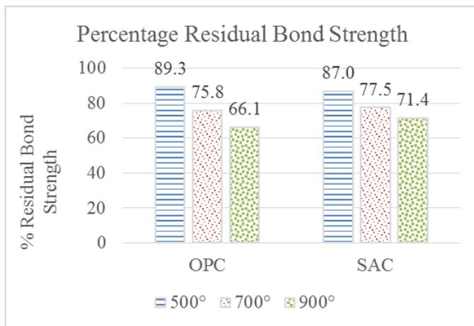
Figure 13: Residual bond strength in SAC and OPC
