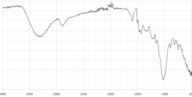
Figure 2. FTIR spectrum of a typical phenolic resin ACP core. (Excelplas1, 2019)
