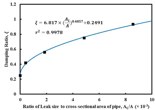
Figure 6. Damping ratios for different leak sizes
