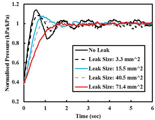
Figure 5. Normalised pressure profile with different leak size.
