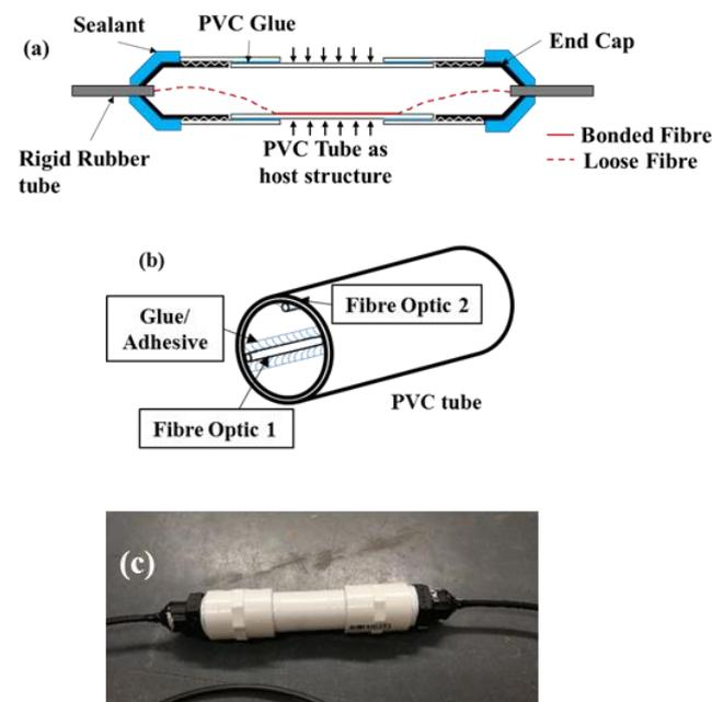
Figure 1(a) Schematic drawing of the prototype submersible optical fibre pressure sensor, (b) depiction of the interior of the PVC tube and (c) depiction of the actual sensor.
