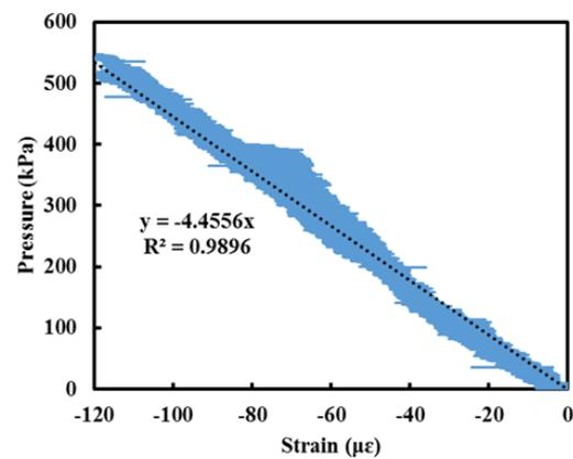
Figure 3. Correlation between the pressure obtained from pressure transducer and strain measured by ODiSI-B.
