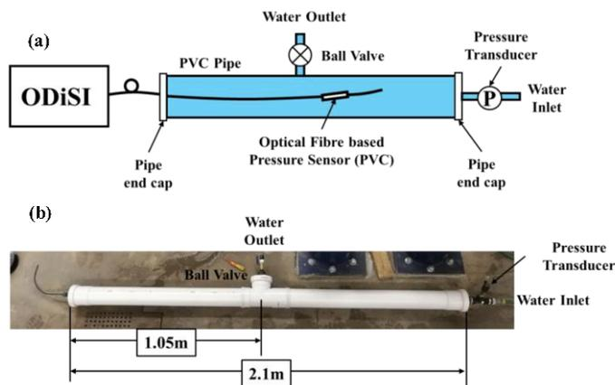
Figure 2(a) Schematic drawing of the experimental set up and (b) the actual experimental set up.
