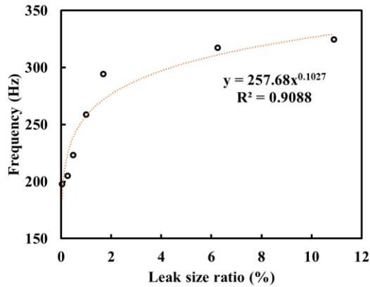
Figure 8. Relationship between the exciting vibration and leak size (in term of % of the cross-sectional area of pipe).
