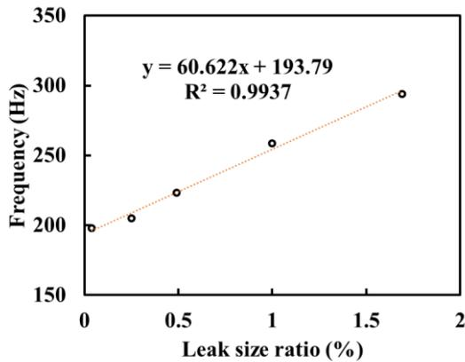
Figure 9. Relationship between the exciting vibration and leak size (less than 2% of the cross-sectional area of pipe).
