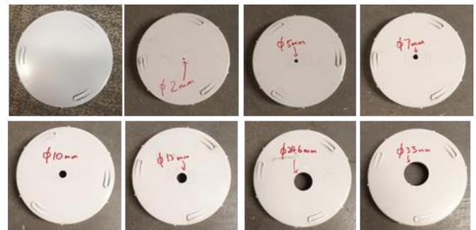
Figure 4. End caps with different drilled diameter at the centre.
