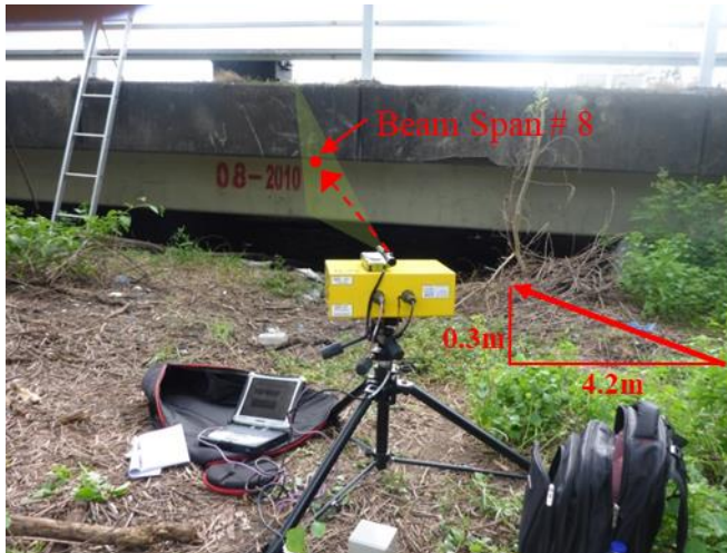
Figure 4. Testing set up of IBIS-S in trestle bridge at Terminal Petikemas
