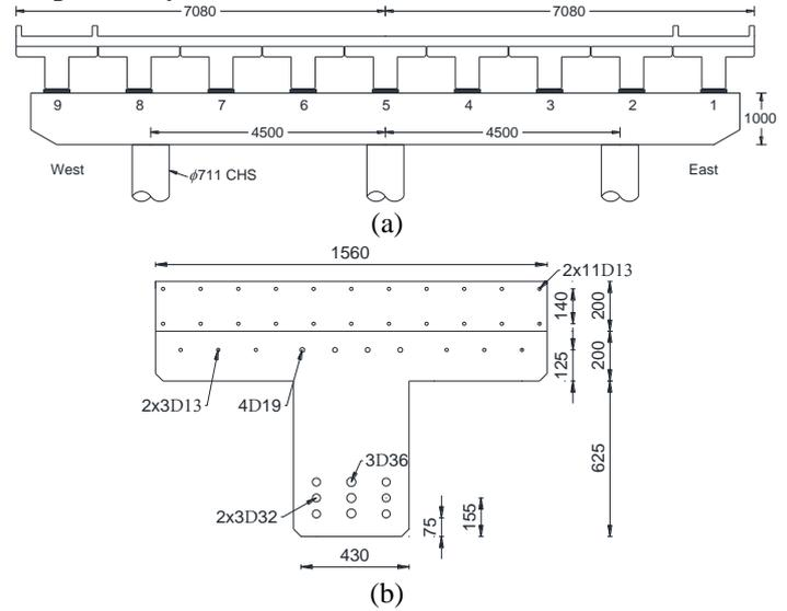
Figure 3. TPS bridge: (a) Cross-section of the bridge looking north; (b) The details for one longitudinal beam
