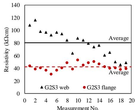
Figure 15. The electrical resistivity of G2S3 in TL bridge
