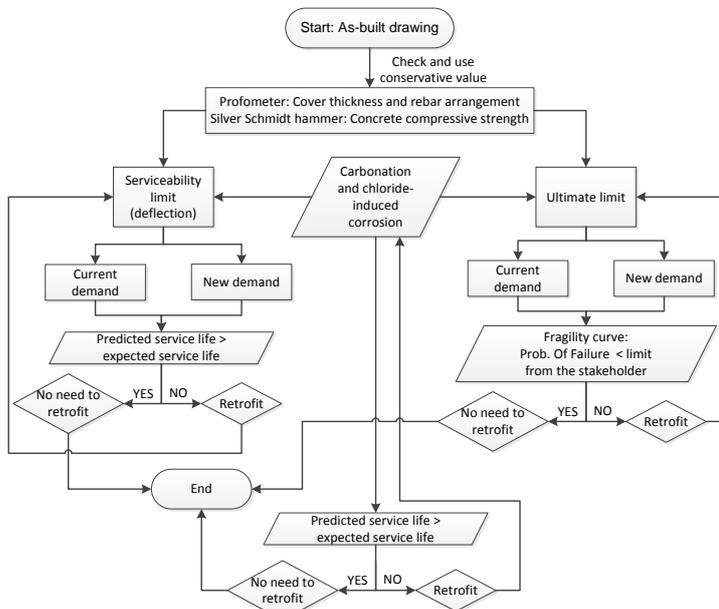
Figure 10. The proposed framework to assess the condition of the existing RC structures
