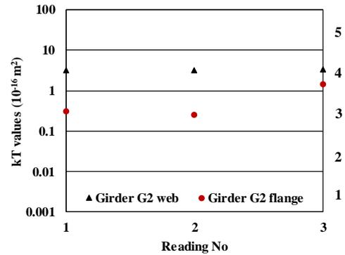
Figure 14. The coefficient of the air permeability for TL bridge
