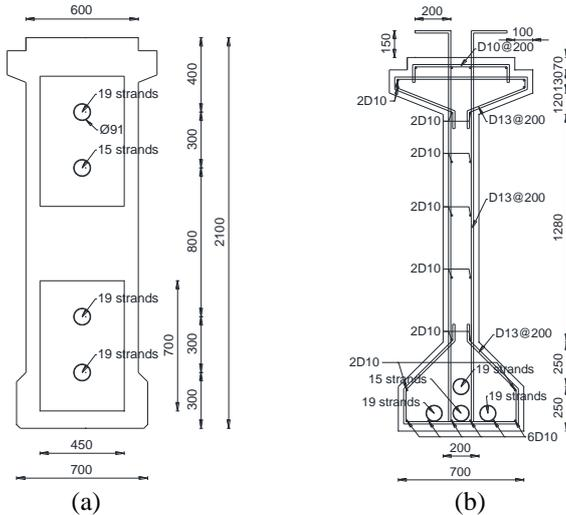
Figure 5. Cross-section of the I girder: (a) at both ends; (b) at the midspan
