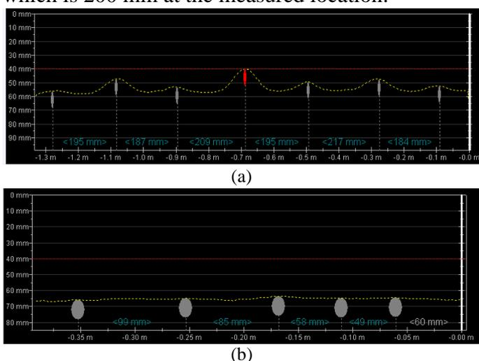
Figure 16. The concrete cover and rebar location measurement using Profometer: (a) Vertical scan for exterior column in TW; (b) Vertical scan for exterior column in TS
