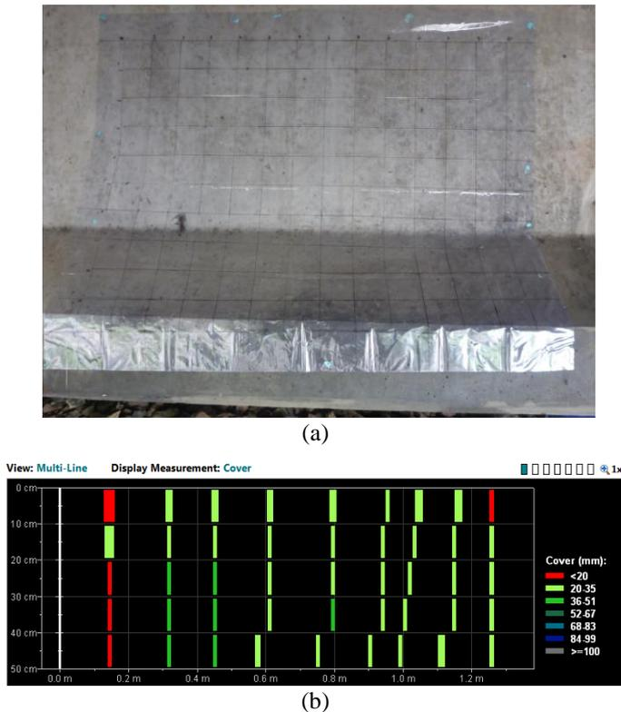
Figure 13. Profometer for longitudinal RC beam at TL bridge: (a) Measured location and (b) Thickness of the concrete cover
