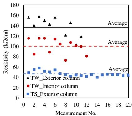
Figure 18. The electrical resistivity for the bridge in Tollway
