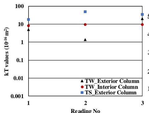
Figure 17. The coefficient of the air permeability for the bridge in Tollway
