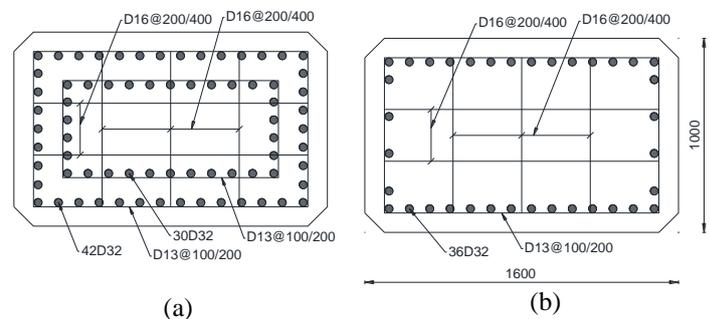
Figure 9. Cross-section of the exterior RC column in Toll Sumo: (a) All columns half bottom; (b) All columns half top
