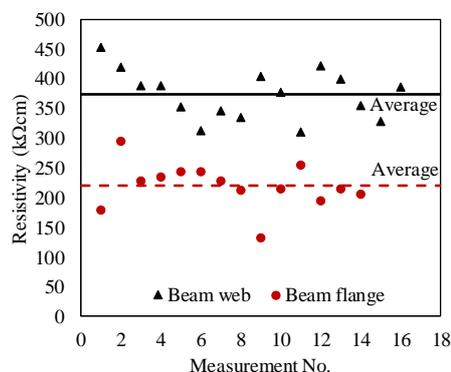
Figure 12. The electrical resistivity of the concrete cover for TPS bridge
