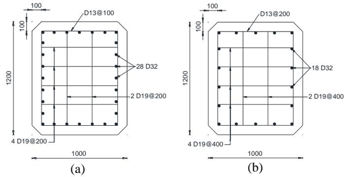
Figure 7. Cross-section of the RC column in Toll Waru: (a) All columns half bottom; (b) All columns half top
