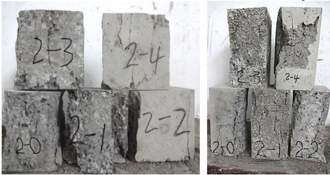
a) Cube compressive test      b) Axial compressive test
