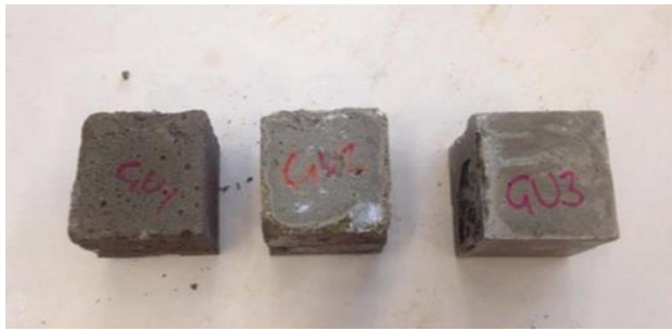
Figure 8. Visual Observation of Efflorescence on Unground Gladstone Specimens for Each Design Mix.
