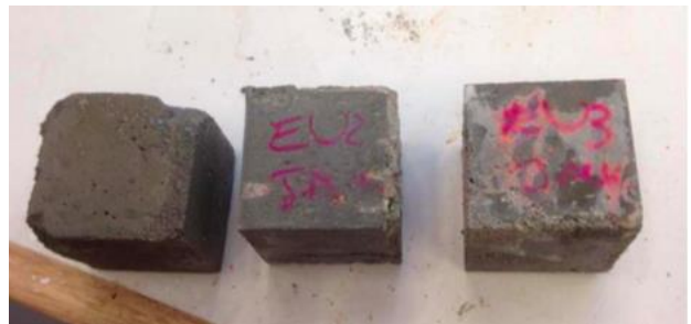
Figure 7. Visual Observation of Efflorescence on Unground Eraring Specimens for Each Design Mix.
