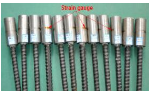
Figure 5 Grouted bolt samples.
