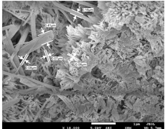
Figure 5. SEM micrograph of cement composite including CNT (Lim et al. 2016)
