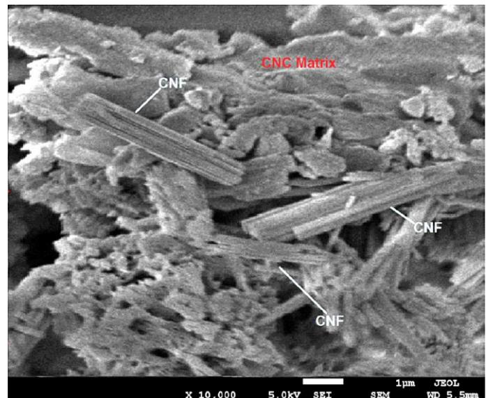
Figure 6. Distribution of CNF within the carbon-neutral cement composite matrix (Lim et al. 2018)
