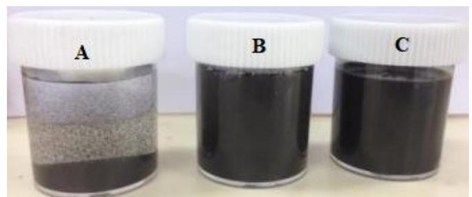
Figure 4. (a) CNT-A dispersed via ultrasonication (without surfactant); (b) CNT-A dispersed via ultrasonication (with surfactant); and; (c) CNT-B dispersed via ultrasonication (Lim et al. 2016)
