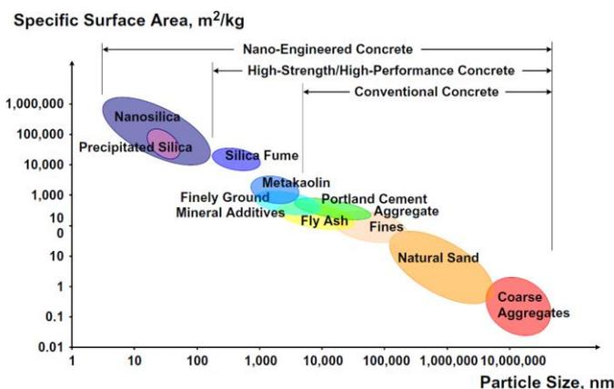
Figure 1. Particle size and surface area distribution of ingredients of concrete [from Sanchez & Sobolev (2010), as adapted from Sobolev & Gutiérrez (2005)].
