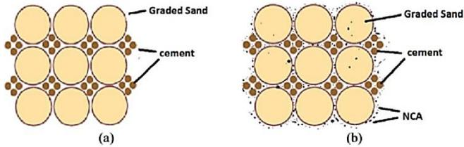
Figure 2. Packing of particles in mortar: (a) without nano-particles; and (b) with nano-particles (Lim et al. 2018).
