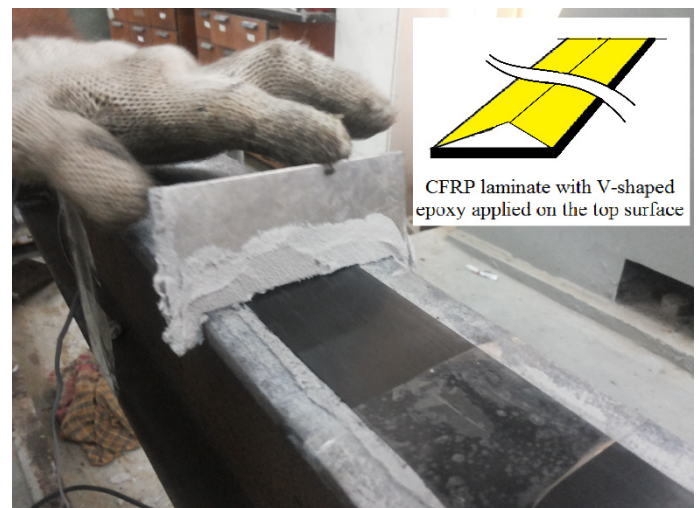
Figure 7. Controlling the epoxy layer thickness of the adhesive and minimizing air voids.
