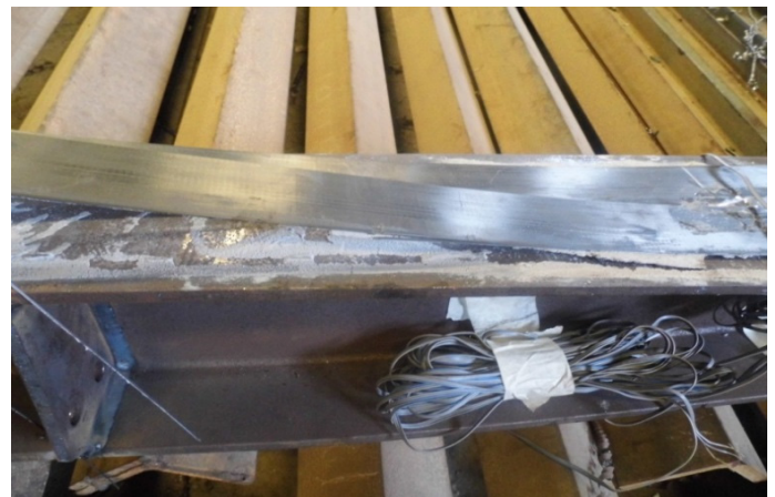
Figure 8. Typical CFRP rupture encountered in testing the beams.
