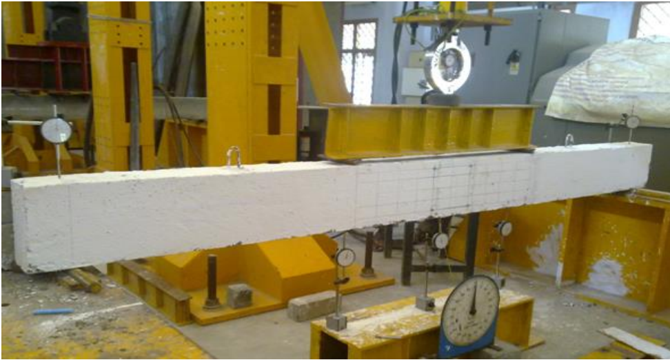
Figure 2. Photographic view showing instrumentation used.
