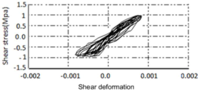
Figure 22. Cyclic Response of CDF1 and CDF2 plotted together.
