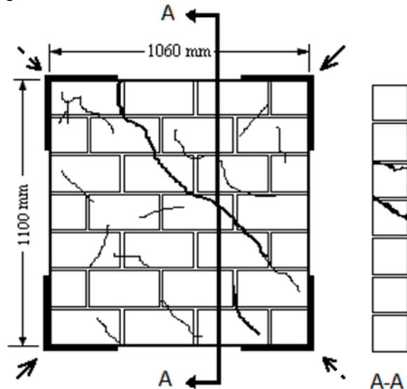
Figure 14. Cracking of CU1.
