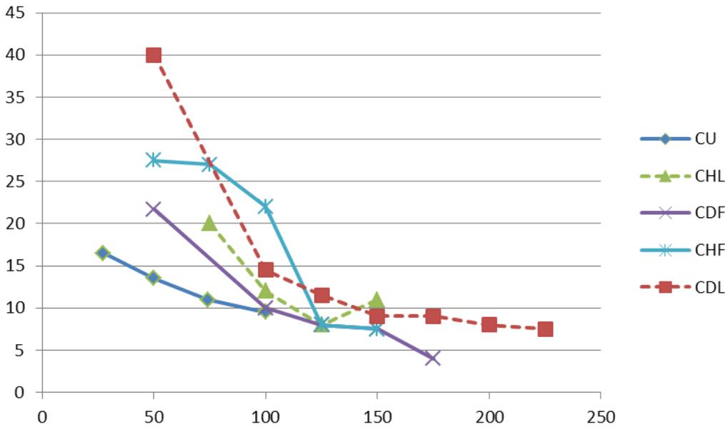
Figure 26. Equivalent Damping Coefficient at Various Load Levels (KN). Dashed are from Santa-Maria et. al. (2004).
