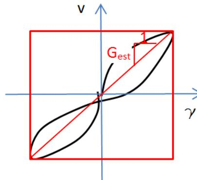
Figure 25. Method of calculation of cyclic shear modulus.
