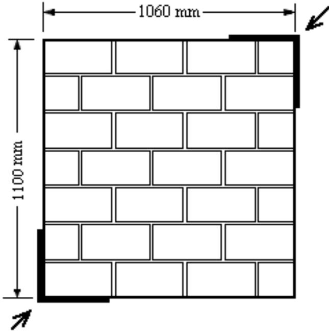
Figure 4. Test arrangement for unreinforced panels under monotonic loading (MU).
