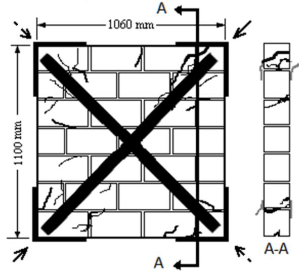
Figure 18. Cracking of CDF4.
