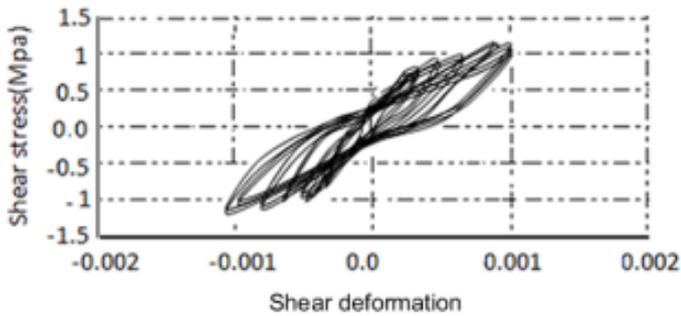
Figure 23. Cyclic Response of CDF3 and CDF4 plotted together.
