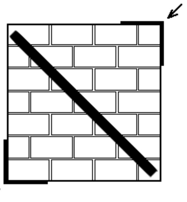
Figure 6. Test arrangement for diagonally reinforced panels under monotonic loading (MD).
