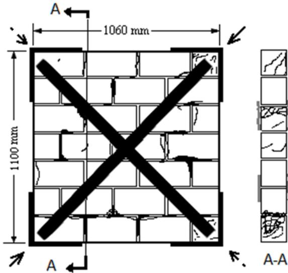
Figure 15. Cracking of CDF3.
