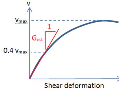
Figure 24. Method of calculation of monotonic shear modulus.
