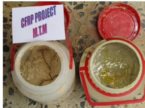
Figure 3. Kimitech Epoxy components (EP-TX).
