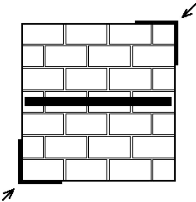
Figure 5. Test arrangement for horizontally reinforced panels under monotonic (MH).
