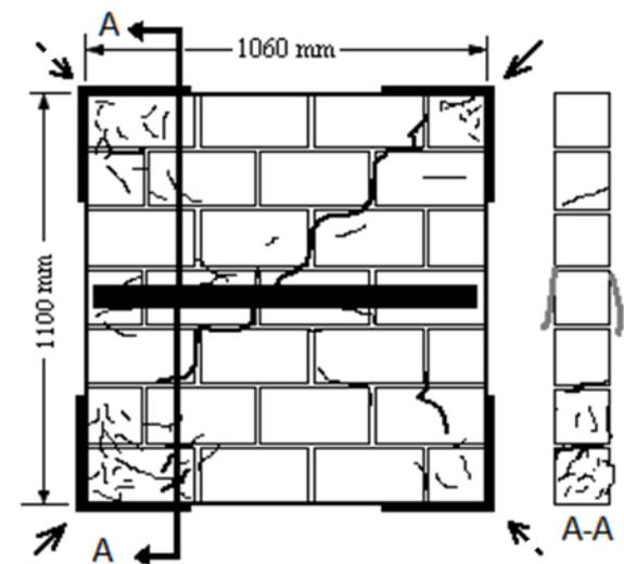
Figure 19. Cracking of CHF1.
