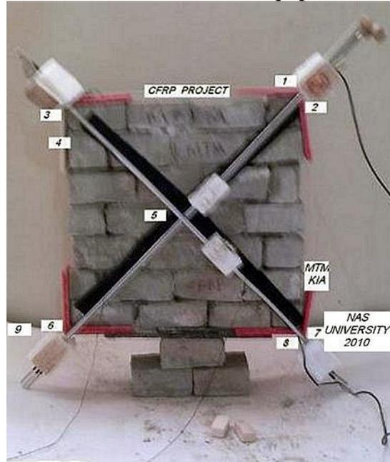
Figure 9. Test Setup for Cyclic Loading Tests. (Key: 1, 3, 7 and 9 are hydraulic rams, 5 is tension rods, 2, 4, 6 and 8 are seats on the edges.)
