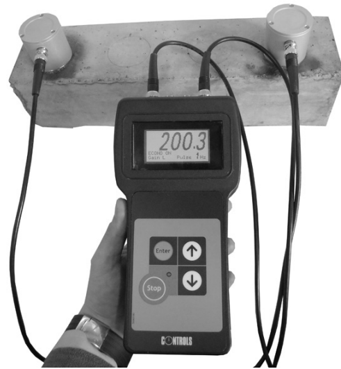
Figure 10. Ultrasonic pulse velocity test apparatus (Adapted from http://www.controls-group.com )
