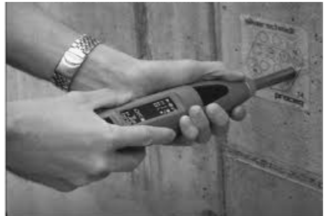
Figure 1. NDT of concrete by Schmidt Rebound Hammer (As adapted from http://www.ntu.edu.sg/ )
