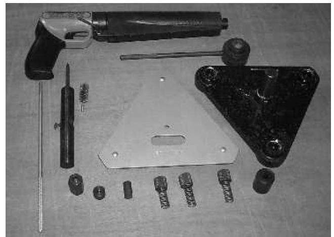
Figure 3. Components of the Windsor Probe System (As adapted from http://www.ntu.edu.sg/ )
