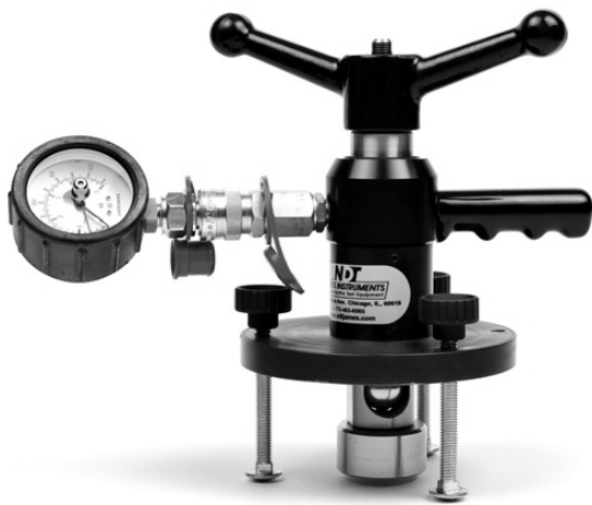
Figure 6. A typical setup of pull-out resistance NDT methods (Adapted from http://www.ndtjames.com )
