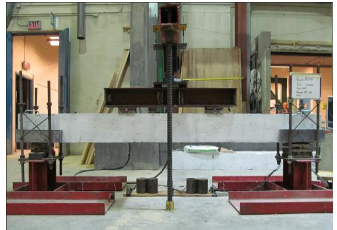
Figure 1. Typical beam specimen prior to testing
