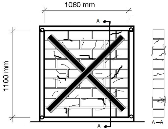
Figure 6. Splitting Crack and Delamination (CFRP-200-2).
