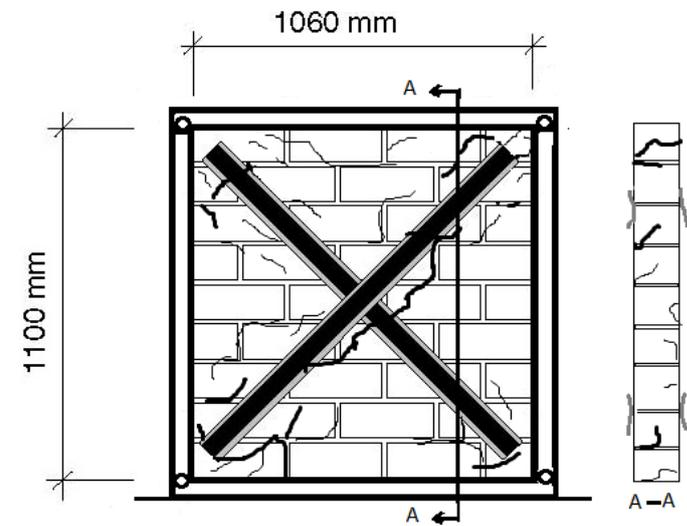
Figure 7. Corner Failure and Delamination (GT-200-2).
