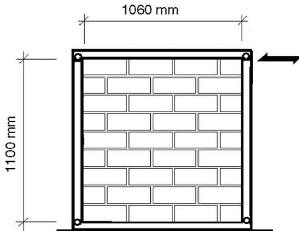
Figure 1. Idealized test arrangement.
