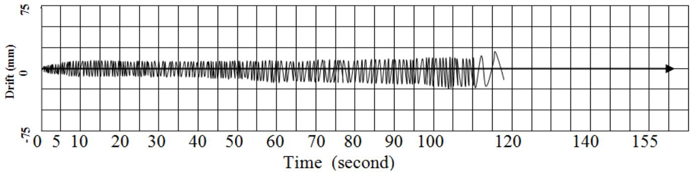
Figure 11. Drift with Respect to Time Under Cyclic Loading of CFRP-100 Panel.
