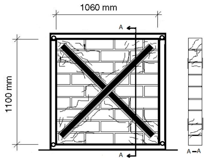
Figure 5. Corner Failure (CFRP-200-1).
