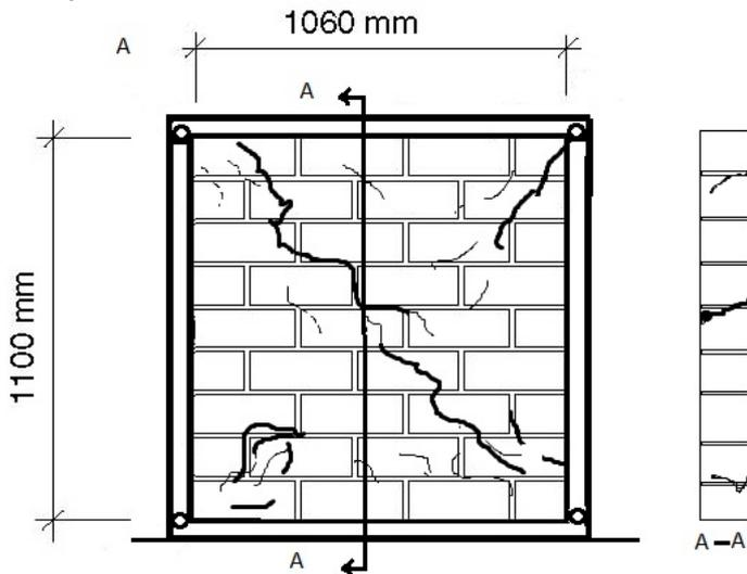
Figure 3. Splitting Crack (URM-1).
