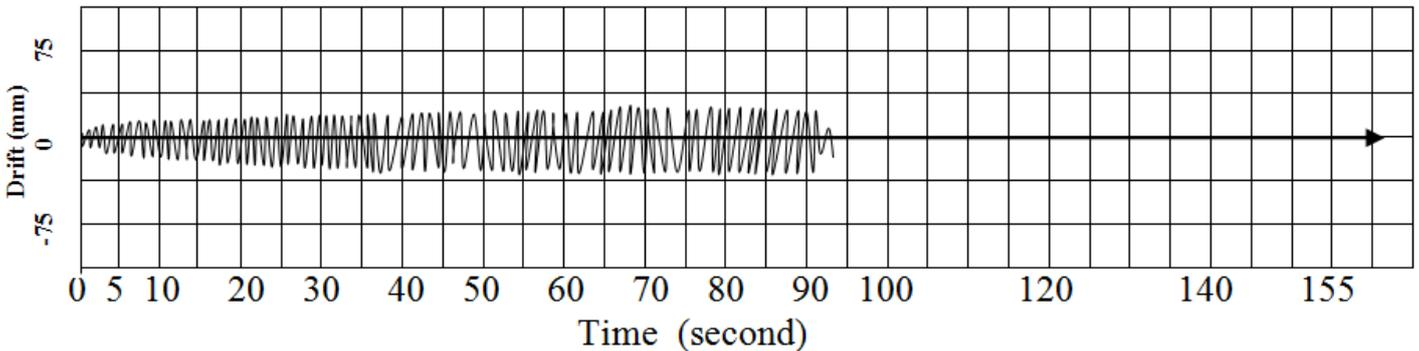
Figure 9. Drift with Respect to Time Under Cyclic Loading of GT-100 Panel.
