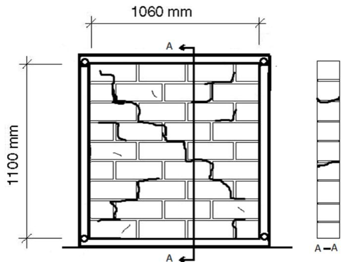
Figure 4. Horizontal Mortar and Splitting Crack (URM-2).
