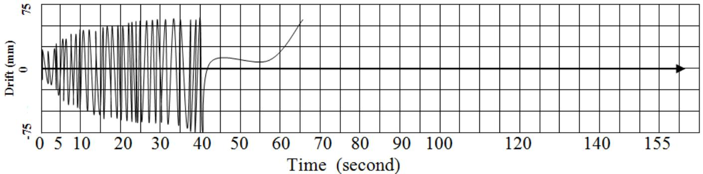
Figure 8. Drift with Respect to Time Under Cyclic Loading of URM Panel.
