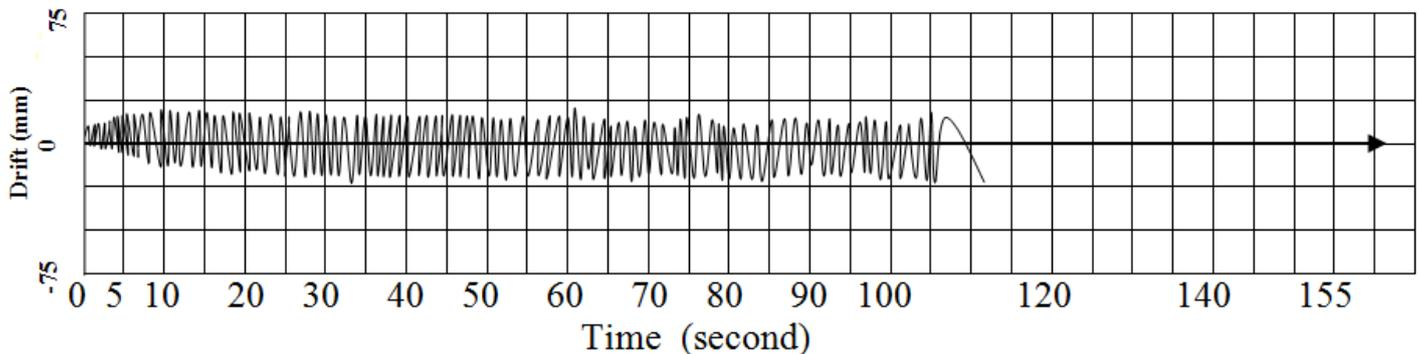
Figure 10. Drift with Respect to Time Under Cyclic Loading of GT-200 Panel.
