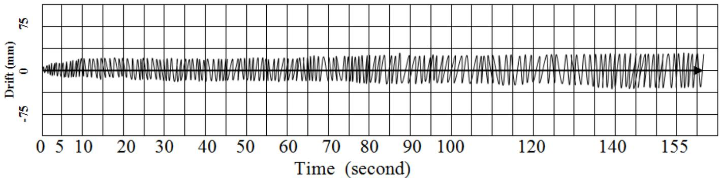
Figure 12. Drift with Respect to Time Under Cyclic Loading of CFRP-200 Panel.
