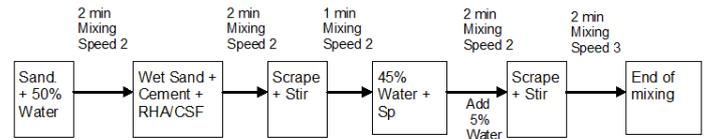
Figure 3: The mixing procedure
