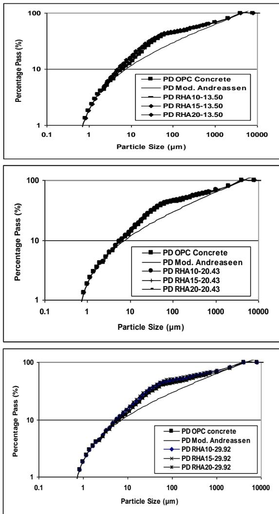
Figure 2: Particle size distribution of mortar incorporating RHA
