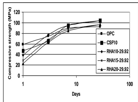
Figure 5: Compressive strength of mortar containing OPC, CSF and several level replacement of RHA
