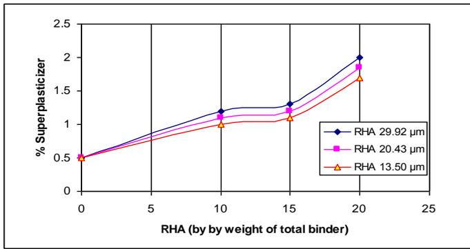
Figure 4: The amount of superplasticizer required for achieving a constant slump flow value of 290 and 300 mm
