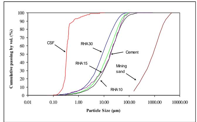
Figure 1: Particle size distribution of RHA, CSF, cement and mining sand
