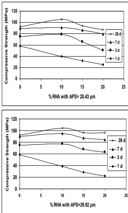
Figure 6: Compressive strength of mortar containing several level replacement of RHA
