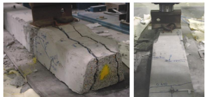
(b) Disintegration and top surface cracks.
