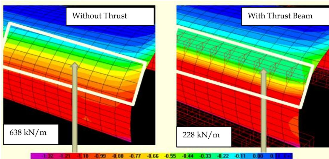
Figure 9 Axial Compression of Steel Structure with and without Thrust Beam
