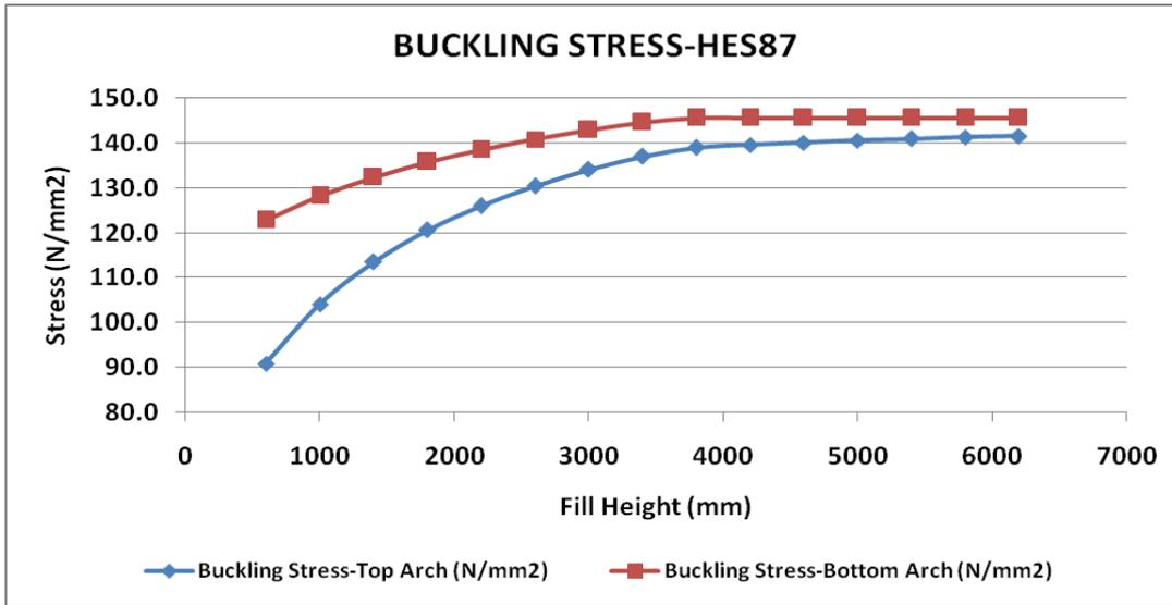
Graph 6 Buckling Failure Stress According to CHBDC, HES 87
