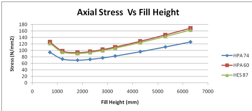
Graph 1 Axial Stresses of Steel Structure According to Ring Compression Theory
