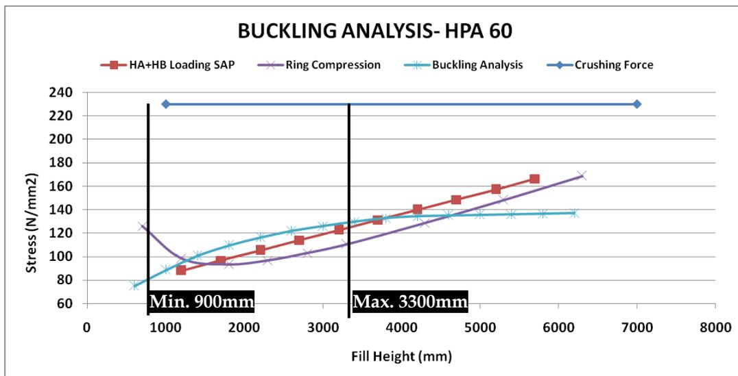
Graph 8 Buckling Failure Stress According to CHBDC, HES 87
