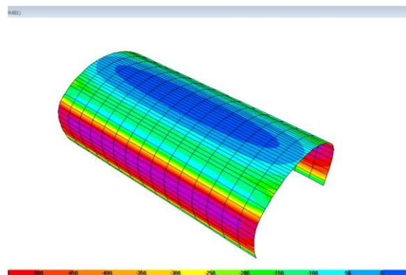
Figure 7 Axial Forces on Steel Arch, SAP2000
