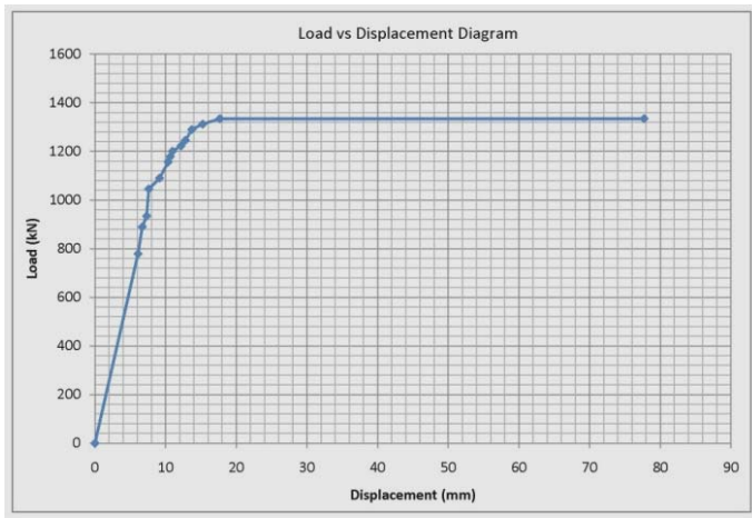
Figure 7. Load-Displacement Relationship for the Five-Column Bent.
