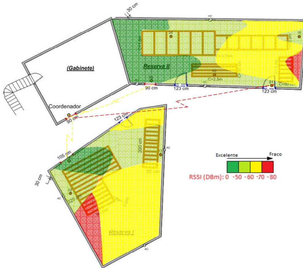
Figure 4. – Final topology and coverage map for the storage rooms of the museum Fortaleza São Tiago.
