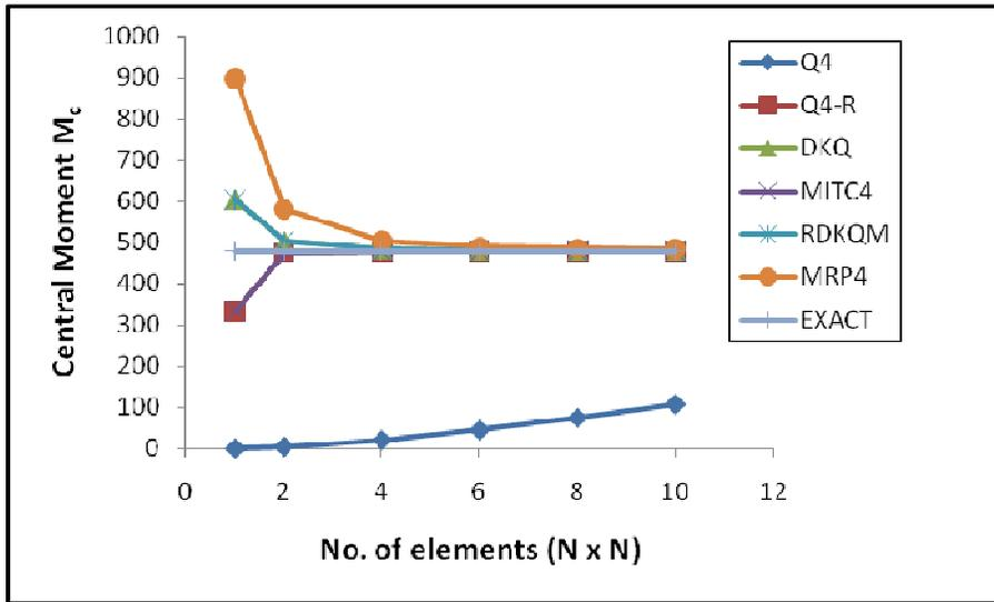
Figure 3: Central moment for a simply supported square thin ( $t/L=0.01$ ) plate with uniform load
