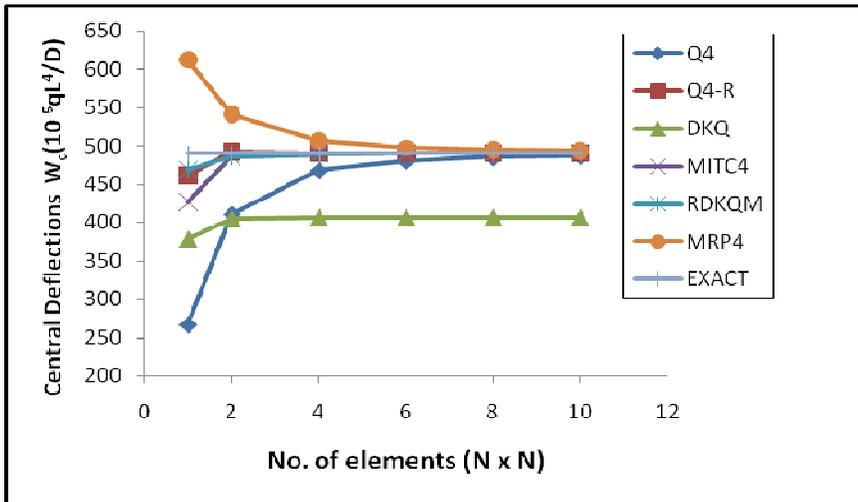
Figure 6: Central deflection for a simply supported square thick ( $t/L=0.2$ ) plate with uniform load
