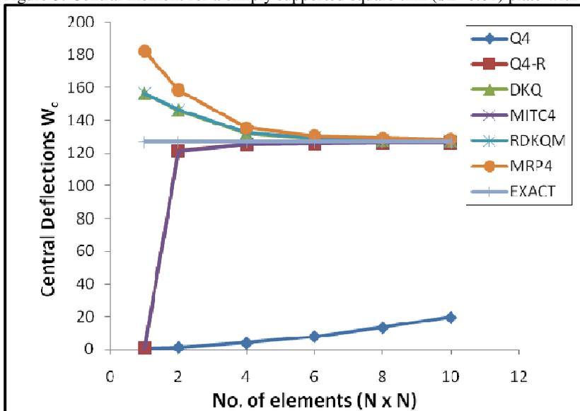
Figure 4: Central deflection for a clamped square thin ( $t/L=0.01$ ) plate with uniform load
