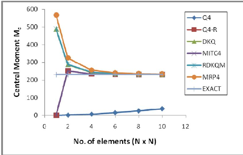
Figure 5: Central moment for a clamped square thin ( $t/L=0.01$ ) plate with uniform load
