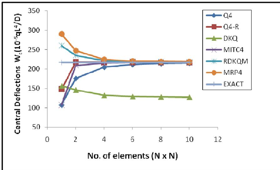
Figure 8: Central deflection for a clamped square thick plate ( $t/L=0.2$ ) with uniform load
