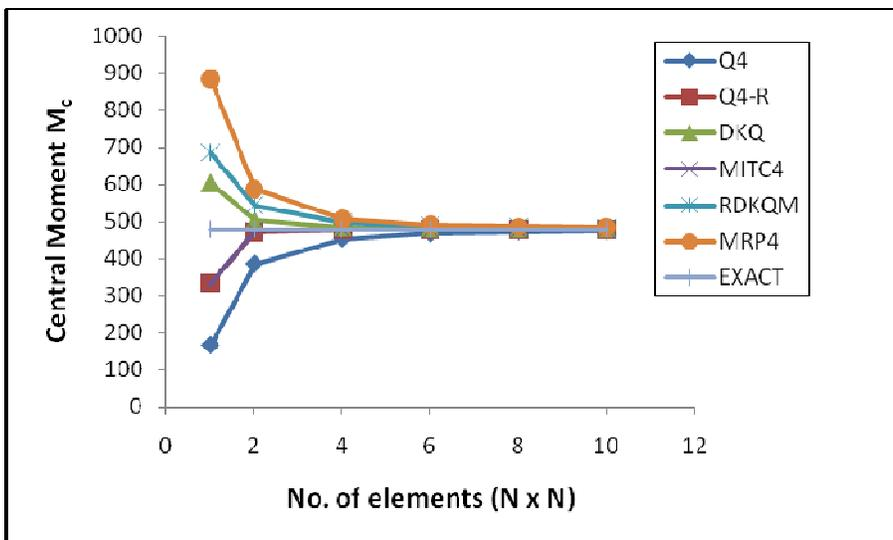
Figure 7: Central moment for a simply supported square thick ( $t/L=0.2$ ) plate with uniform load
