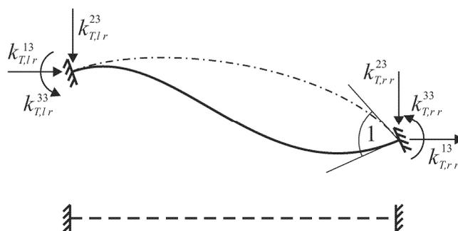
Figure 3. Negative influence line for the bending moment at the right end of the deformed element.
