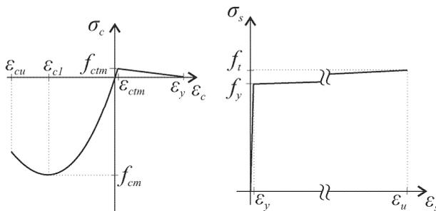
Figure 5. Assumed stress-strain relation for concrete and reinforcement.
